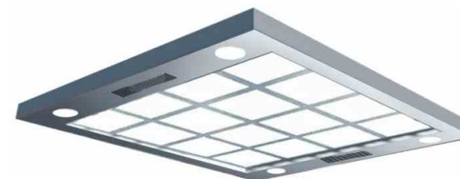
SC-112(Optional) Height 100mm; Hairline ST/ST (Option: Mirror ST/ST) + Acrylic panel + LED lamps; Direct ventilation; Emergency exit Available
