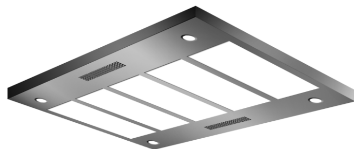
SC-104(Optional) Height 100mm; Hairline ST/ST (Option: Mirror ST/ST) + Acrylic panel + LED lamps; Direct ventilation; Emergency exit Available
